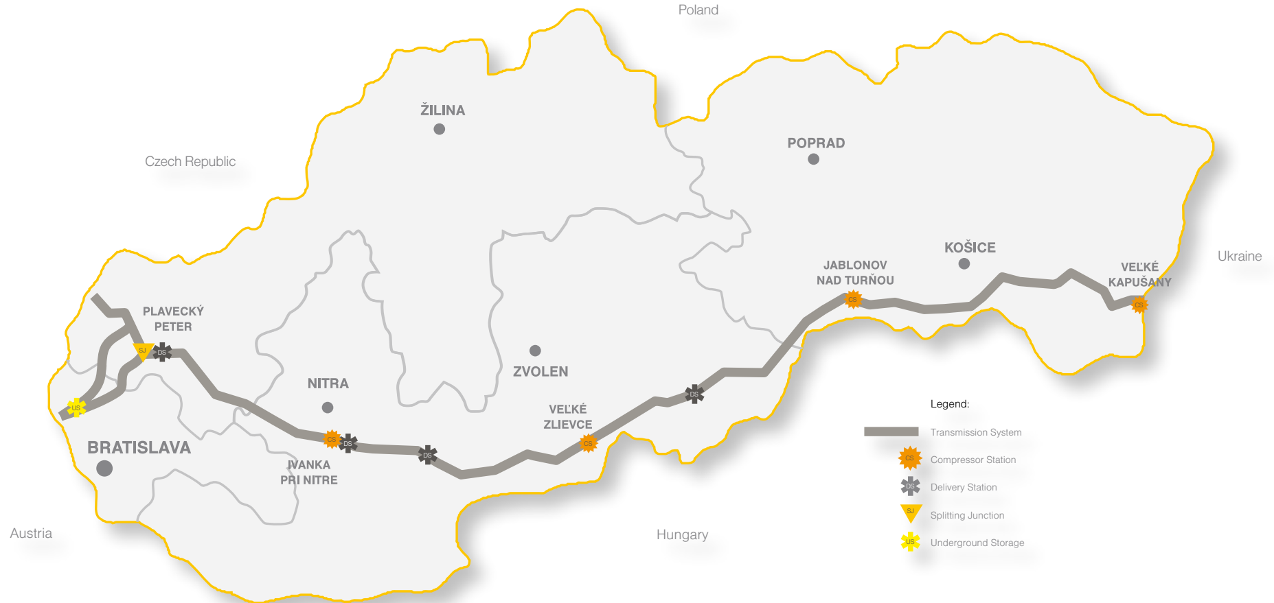
The Transmission System operated by Eustream
