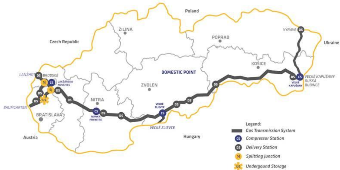
Picture 2: Structural representation of Slovak natural gas transmission system with an appropriate level of detail
